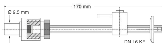
Fig. 4: Test leak with pin housing and VCO connection
